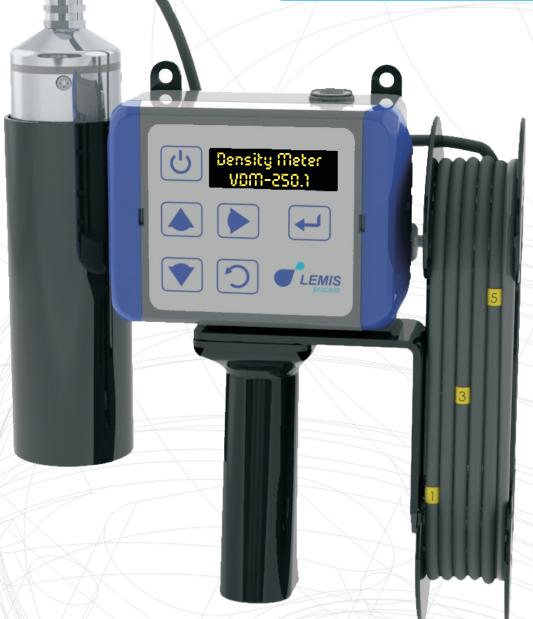
**Portable Submersible Density & Viscosity Meter**
